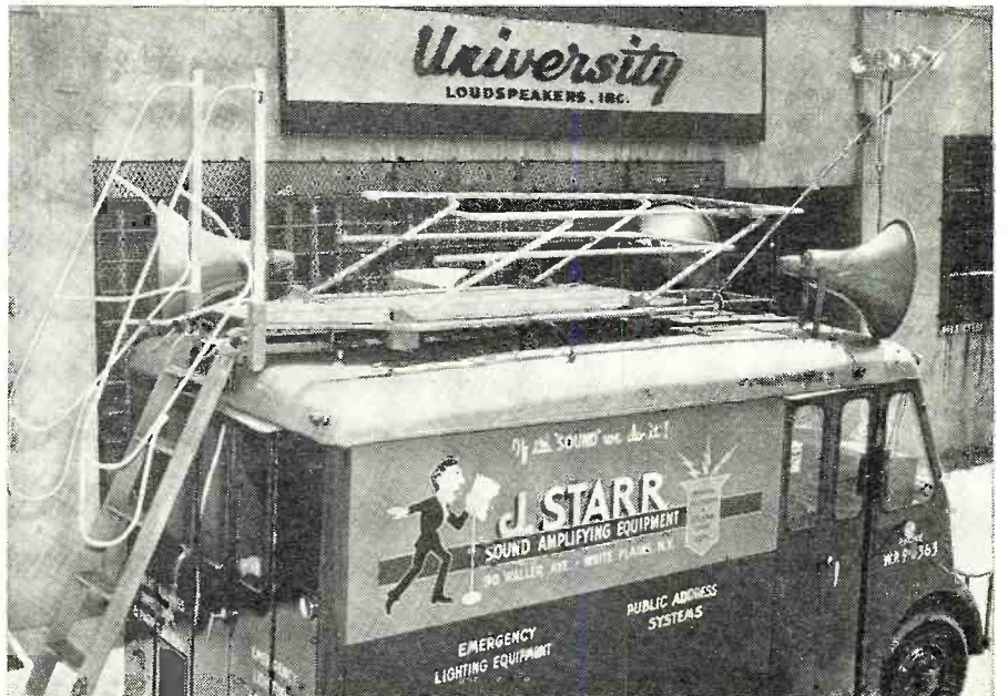
Fig. 12. Closeup view of top of sound truck with announcer's stand partially collapsed.
