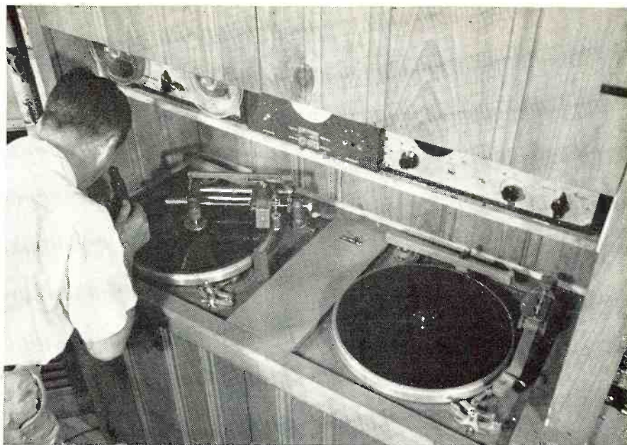
A bird's eye view of the two disc recording and playback channels. Ample storage space for the processed transcription discs is provided in the cupboards below.
